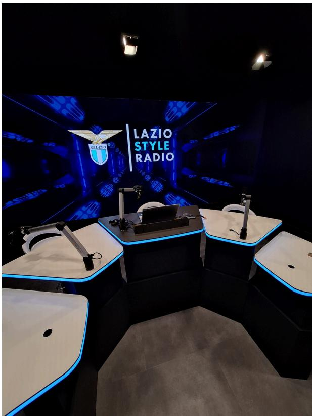
Each announcer station is motorized and independently height-adjustable, allowing the desk to be adapted to different operational needs, both in a seated and standing configuration. This flexibility ensures ergonomic comfort and aesthetic consistency in any production context.
